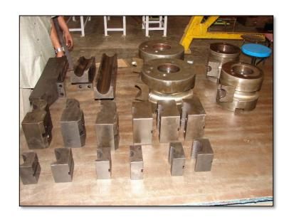
♦ We have manufactured tooling for split type construction tooling, Booster bending applications, we have manufactured tooling from Ø5 mm to Ø127 mm and CLR from 10 mm to 350 mm.
