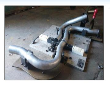
These fixtures are manufactured for holding of bent pipes for cutting operation these are designed to work with down saw cutting machines main feature of these fixtures is repeatability in holding and positioning of pipe for precision cutting in accuracy of plus or minus 300 microns.
