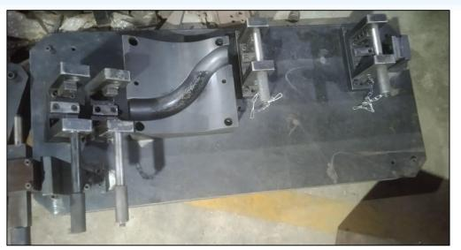
▶ It is designed for checking of bend pipes this fixture consists of elements for pipe position checking in the straight portion even with complex bend angles ,also it features bend profile templates at bend radius for complete profile checking of pipe
