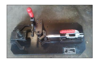
**☼**These fixtures are manufactured for holding of sheet metal assembly's for final operations such as drilling or reaming operations these fixtures have plp location and clamping and also equipped with jig bushes for tool guideing to ensure proper accuracy and positioning
