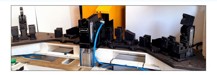
This fixture is specially designed for the handlebar pipe of two-wheelers. It has a pneumatic clamping system and a mechanical stopper arrangement to observe the pipe length after swaging. The fixture has the capability to clamp two handlebars at the same time for the cutting operation on the specific SPM.
